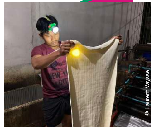
Visual inspection of a freshly laminated rubber sheet by a tapper
